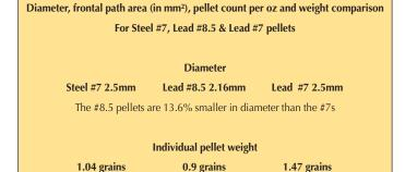
The steel #7s have a 35% larger frontal area then the lead #8.5s, but are only 15.5% heavier. Conversely the lead #7s have the same frontal area but are 41.5% heavier than the steel #7s.
