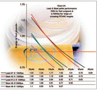
the idea is that this will be sufficient to deliver in at least a like for like manner when compared to the lead #7.5 pellet at the same velocity of 1300fps. To enhance steel #6s further, it has also been suggested that a velocity hike (such as to 1500fps) over and above the usual higher speed target loadings of 1300fps would be sufficient to match up with lead #7s. Unfortunately, it is here that the Steel #6 concept falls into error.
