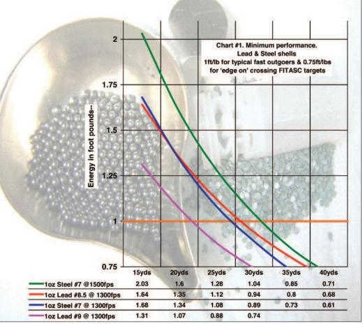
but steel #7s fall behind the 1300fps lead #8.5 pellets after 20 yards. This is despite the higher initial energy of the larger and heavier steel #7 pellets.
